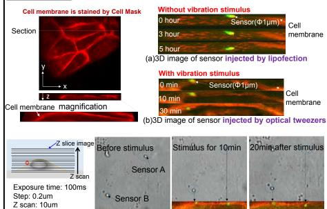
Conclusions We succeeded to adhere the sensor to a cell selectively through optical control. We also achieved rapid sensor injection (approximately 30 min) into the cell by applying local mechanical stimulus using optical tweezers with amplitude of 4 µm and frequency of 1Hz.
