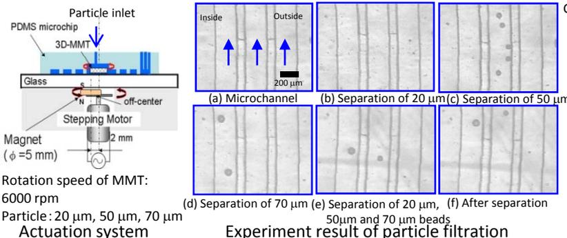
Improvement of filtration efficiency by MMT was confirmed.
