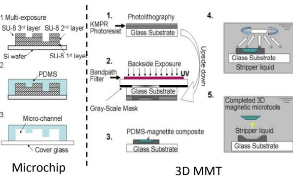
Fabrication process of microchip and 3D MMT
